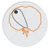
Figure 5. R500 5GHz Elevation Antenna Patterns
