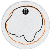
Figure 4. R500 2.4GHz Elevation Antenna Patterns
