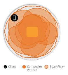
Figure 2. R500 2.4GHz Azimuth Antenna Patterns
