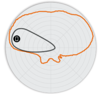
Figure 5. R610 5GHz Elevation Antenna Patterns
