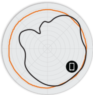
Figure 2. R610 2.4GHz Azimuth Antenna Patterns
