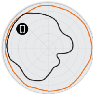
Figure 3. R710 5GHz Azimuth Antenna Patterns
