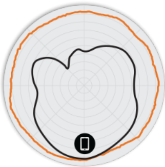
Figure 2. R710 2.4GHz Azimuth Antenna Patterns
