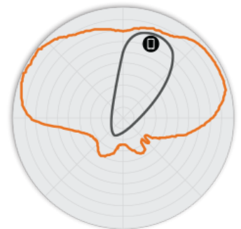
Figure 5. R710 5GHz Elevation Antenna Patterns
