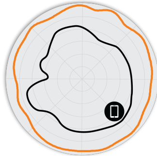
Figure 3. R650 5GHz Azimuth Antenna Patterns
