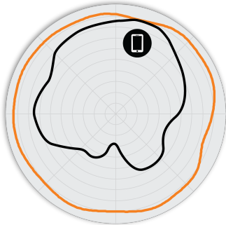
Figure 2. R650 2.4GHz Azimuth Antenna Patterns
