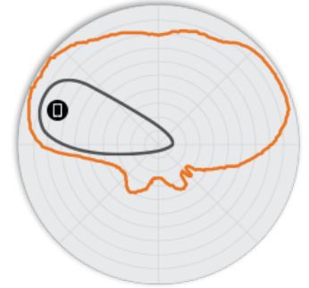
Figure 5. R750 5GHz Elevation Antenna Patterns
