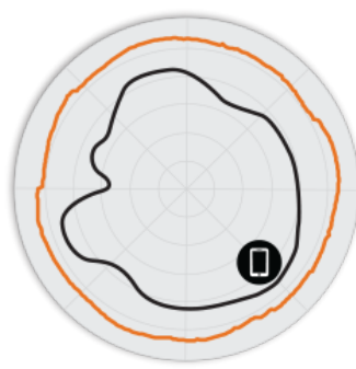
Figure 3. R850 5GHz Azimuth Antenna Patterns
